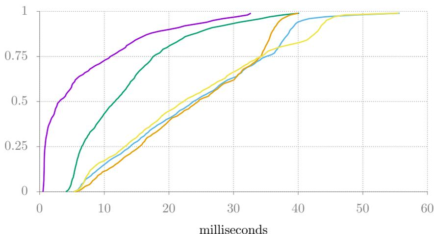
In this graph, we show the processing time CDF of 1000 sequential accesses to a stock Mac OS X “Lion” Apache server, both as a static file (in red) and stub CGI script (in green). The mean processing time for the former, our baseline, is 5.207 ms; the mean processing time for the latter, which demonstrates the overhead in spawning and communicating with a child CGI process, is 13.8 ms—over two times the baseline.
