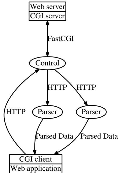
The control process reads requests from the CGI server, pushing data per request into the pool. When the pool parses and validate pairs, it passes them to the *kcgi* CGI client, which builds up a request object. Finally, when all pairs have been read for a given request by the *kcgi* CGI client, the request object is passed to the web application.
