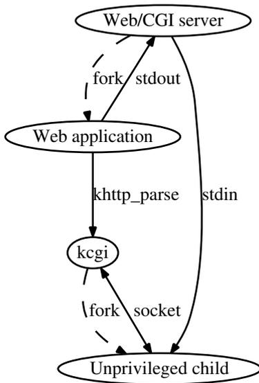
In the current *kcgi* implementation, the `khttp_parse(3)` function is invoked by the web application as early as possible. The function then creates a socket pair and spawns a child, with an option (via the extended `khttp_parsex(3)`) for the child to scrub its parent’s memory. The socket pair is one-directional, with the parent reading and the child writing. The child process inherits its parent’s standard input, which it uses to read input from the CGI server.
